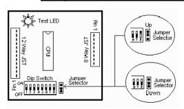
"UP" for active LOW Open Collector Ticket Drive Output (Used with DL4 Ticket Dispenser).
